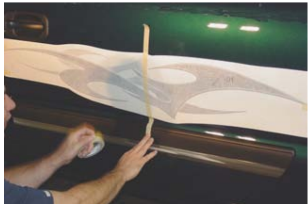
2. Apply a strip of tape vertically through the center of each component and lightly tape each end of the graphic panel to the vehicle.
