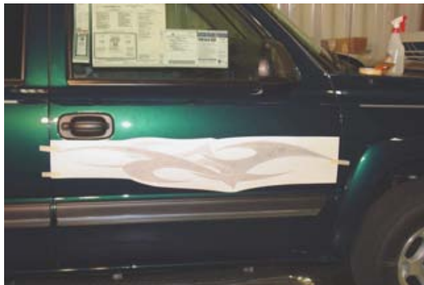
1. Tape the graphic onto the side of vehicle to determine exactly where you want the graphic installed.
