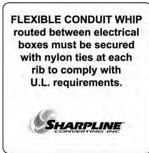
The Flexible Conduit Whip Label reminds installers that it must be secured with nylon ties at each rib to comply with U.L. requirements.
