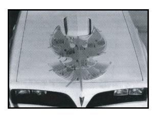
2. To the right of centered strip of making tape, lift graphic away from backing paper and cut backing paper off with scissors or very sharp blade.
