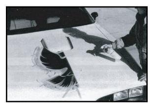
4. Carefully lay graphic onto paint surface and squeegee stroke decal with overlapping motions from the center of body out towards wing tips. Repeat the first three steps for the opposite side of the decal before proceeding to the next step.
