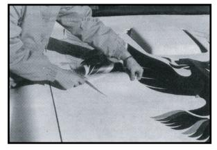
8. Squeegee each wing down, moving from the center of the wing towards the outer edge.
