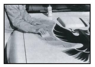
9. Remove masking paper, and hood bird is complete. All additional parts such as sail panel birds, shaker scoop decals, fender names, and spoiler name may be installed using the same procedure.
