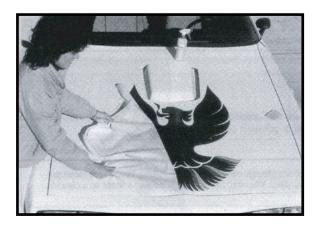
6. With masking tape, position wing tips into place.
