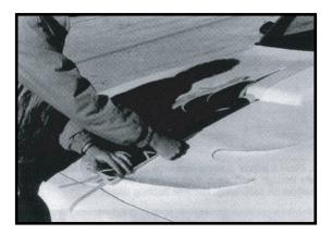
3. Lubricate surface of vehicle with Easy-On application solution so that graphic will be easier to work with.
