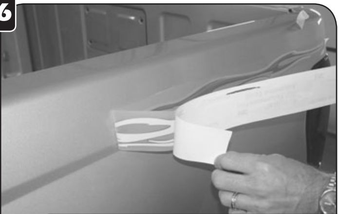
Remove the masking tape 'hinge' from the center of the graphic component. Then remove the remaining liner paper (backing paper) from the graphic component and discard. Squeegee the remaining half of the panel onto the vehicle utilizing the same method described in step #5.
